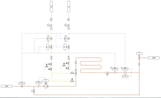
$\mathrm{CO_2}$  and  $\mathrm{N_2}$  is injected into the beer via the GDI gas injector developed by corosys. The gas injector splits the gases into very small bubbles and ensures that the  $\mathrm{CO_2}$  completely dissolves in a very short time. The system works without using a static mixer.
