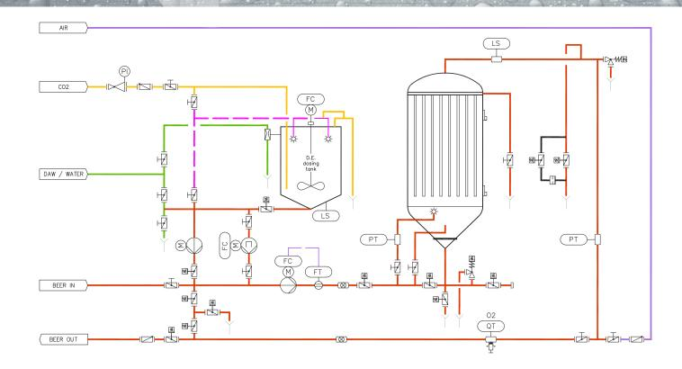
To achieve excellent filtration results stainless steel filter candles are used as the carrier for the DE (Kieselguhr). The candles are first covered with coarse and subsequently with finer DE type.
