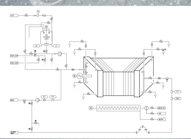
To achieve excellent filtration results stainless steel filter elements (stainless steel frames) are used as the carrier for the DE (Kieselguhr). The filter elements are first covered with coarse and subsequently with finer DE type.
