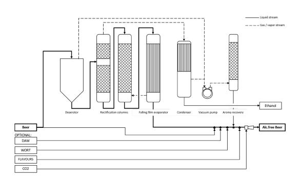
During de-alcoholization of carbonated products, degassing takes place in a first process step.
