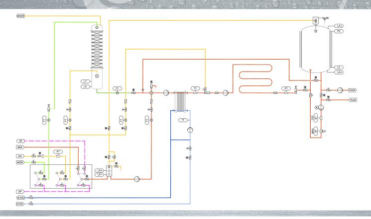
The beverage water is degassed in a column under normal pressure by stripping with  $CO_2$  to residual oxygen values below 50 ppb. Here, the water is pre-carbonised with approx. 2 g/l  $CO_2$ .
