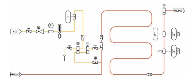
$\mathrm{CO}_2$  is injected into the beer via the GDI gas injector developed by corosys. The gas injector splits the  $\mathrm{CO}_2$  into very small bubbles and ensures that the  $\mathrm{CO}_2$  completely dissolves in a very short time. The system works without using a static mixer. The homogeneous dispersion and the absence of gas bubbles can be monitored by a sight glass situated at the outlet of the dissolving path.
