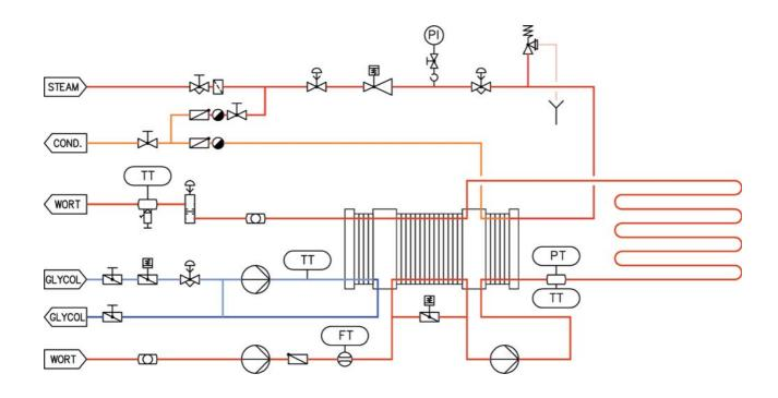
The wort is gently heated up to the sterilization temperature regeneratively and then via steam. Then it is flowing through a holding pipe to keep the sterilization temperature for a specified time and to reach the required germ reduction. After this the wort is cooled down regeneratively and further cooled with glycol or ammonia.
