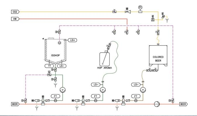
The flow of product is measured by an electromagnetic flow meter at the inlet of the system. The system doses the additives according to product flow and in a fixed rate given by the recipe for malt extract, hops products, flavours or enzymes. The flow of additives is controlled by frequency controlled metering pumps or by control valves.
