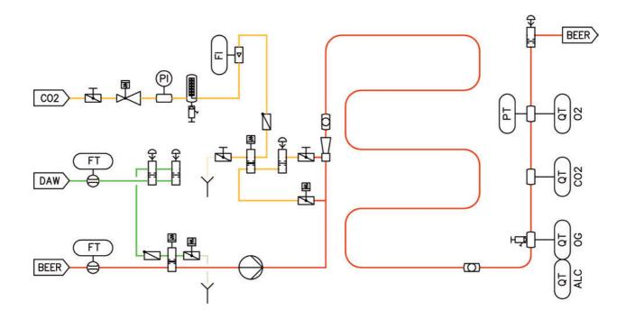
The flow of beer and water is measured by electromagnetic flow meters at the inlet of the system. Two parallel control valves of different size adjust the flow of deaerated water as a percentage of the beer flow. The follow-on centrifugal pump pumps the beer through the carbonization to the BBT and at the same time mixes beer and water homogenously.
