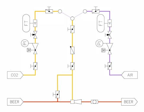
Like our carbonation system CCS, the corosys gas injector GDI is the heart of the carbonation device CCS M. The gas injector splits the  $\mathrm{CO}_2$  into very small bubbles and ensures that the  $\mathrm{CO}_2$  completely dissolves in a very short time in the following pipe line. The system works without using a static mixer.
