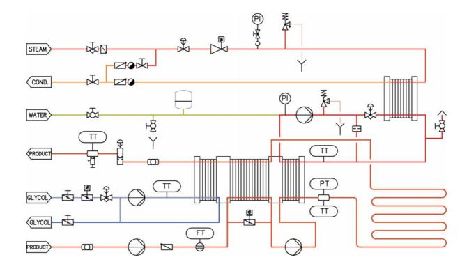
The product is gently heated up to the pasteurization temperature regeneratively and then via a hot water circuit. Temperature and flow are controlled to keep the pasteurization units within very narrow limits. Then the product is cooled down regeneratively and further cooled with glycol or ice water after passing the holding pipe.
