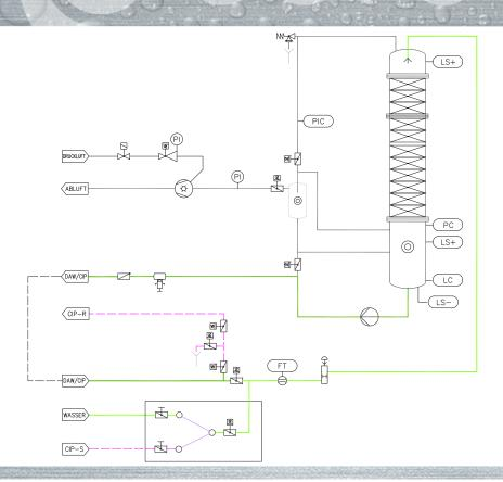
The water is distributed homogeneously to the structured packing at the top of the column. It slowly flows downwards through the structured packing. An excellent distribution of the water in the column is ensured by the high-performance structured packing. The resulting enlargement of the contact surface of water causes an optimal removal of oxygen. Due to the combination of two degassing steps operated at different pressures, lowest oxygen values are reached.
