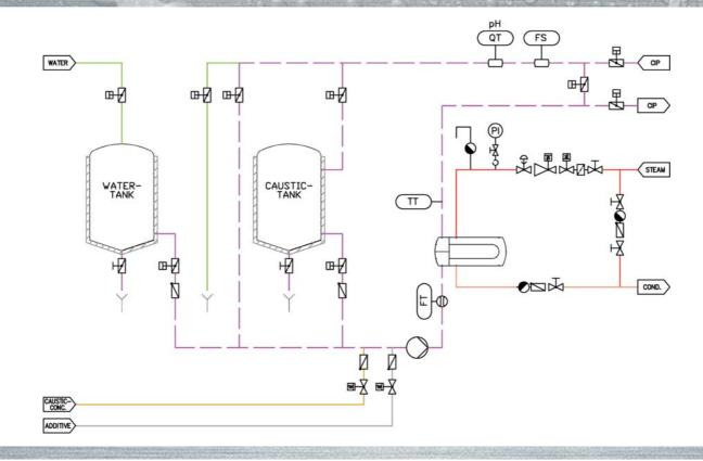
The CIP plants are designed and equipped with tanks for storage of cleaning agents or designed for lost CIP with one or more cleaning circuits, depending on the cleaning task. Different cleaning circuits and programs can be stored with their specific parameters and run fully automatically. Flow velocities are optimally adapted to each cleaning task and the system dimensions.
