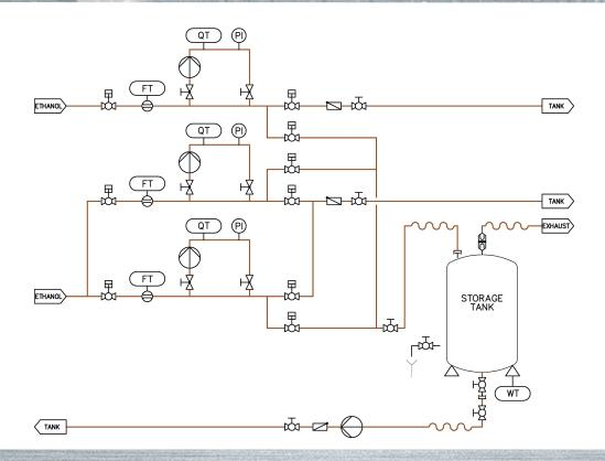
A Coriolis mass flowmeter measures the mass flow of ethanol in the main stream. The alcohol concentration is measured in a bypass by an extremely precise density meter of Anton Paar, Graz, Austria. The signals of both instruments are evaluated by a flow computer. The volume of the alcohol / water mixture and the volume of pure ethanol at a reference temperature of 20 °C is calculated, counted and stored.
