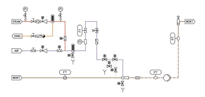
Sterile air or oxygen is injected into the wort via the GDI gas injector developed by corosys. The gas injector splits the air / oxygen into very small bubbles and provides quick and complete saturation. The wort pipe between wort cooler and fermenter functions as a holding pipe.
