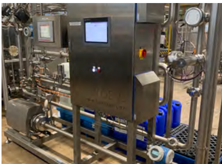
The CCS carbonation system offers a wide range for CO 2 dosing for both beer and mineral water
